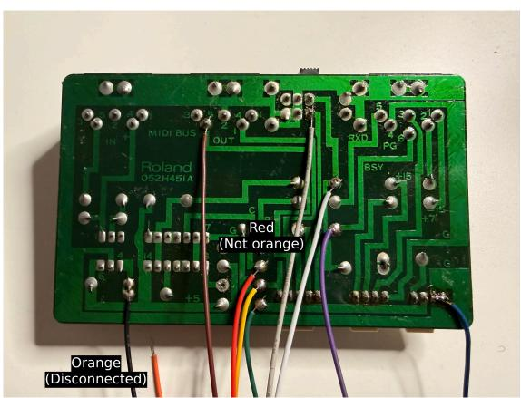
5. Solder the orange cable from the 10-pole cable bundle to the yellow cable that was disconnected from the 5-pole cable bundle in step 2, use heat-shrink wrap or electrical tape to enclose the point of connection.
