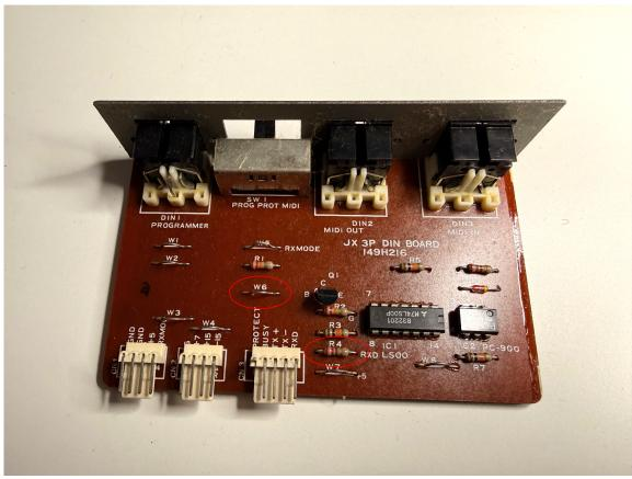
4. Now solder each of the 9 wires of the supplied 10-pole cable bundle (rainbow coloured) at the locations indicated in the PCB layout below:
