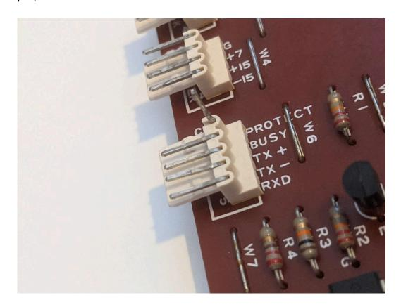
2. Cut and strip or otherwise remove the yellow wire from the 5-pole cable bundle that connects to CN3 (the pin header modified in the previous step).
