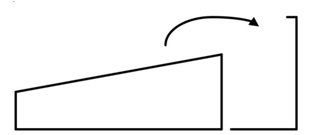
Partially remove the keyboard outside the case. You do not have to unplug the cables connected to it, as you only need to move it just enough to reach the firmware EPROM on the mainboard. Avoid touching the power supply (capacitors can still be charged after power is disconnected).
