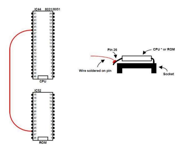
Pay attention to the orientation of pin 1 when inserting the new ROM. Reversed insertion of the IC into the socket could damage the IC and other components in the JX-3P.
